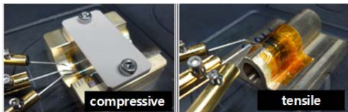
Figure 3. Electrical characterization of LTPS TFTs under compressive or tensile strain. Each cylindrical metal tube has various radiuses such as 2 to 7R (mm).
